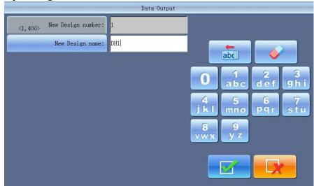
The system uses the design name in memory as the default name for the design in disk. Use keyboard on the right to change the name.
