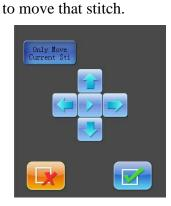
When user presses "Only Moves Current Sti"down, the absolute position of all of the stitches behind current stitch will keep still. If that key flicks, the relating position of current stitch and all of the stitches behind it will keep still, which means that, at the same time of moving the current stitch, the absolute positions of stitches behind it are changed correspondingly.
