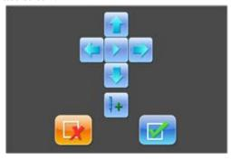
Users need to locate cursor to the right position by clicking direction keys. Press **1** to insert a stitch to that point; then user can move the cursor add more stitch form.
