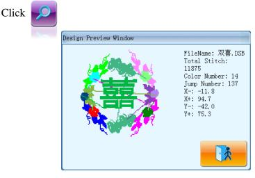
The system loads the data from the disk and displays the design's image according to a certain ratio. At the same time the design's information and color-changing number will be shown in the information area.
